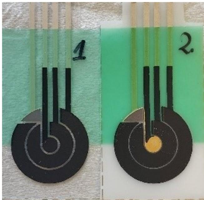
**Figure 9.** Screen-printed electrodes purchased from Donflex. Counter and working electrodes of carbon and a pseudoreference of silver. The right electrode (2) has a central working electrode with electrodeposited gold.
